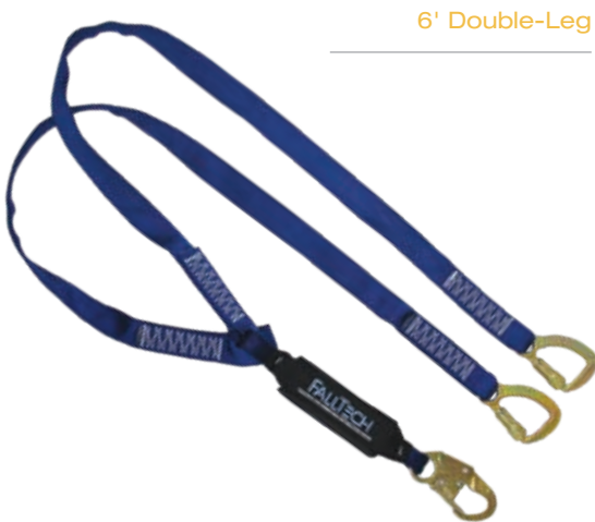
100% tie-off WrapTech® Tie-back lanyard with ViewPack® external energy absorber, jacketed dual-layer polyester web legs, 5,000 lb. gated carabiners for tie-back anchorage and steel snap hook for harness attachment.
